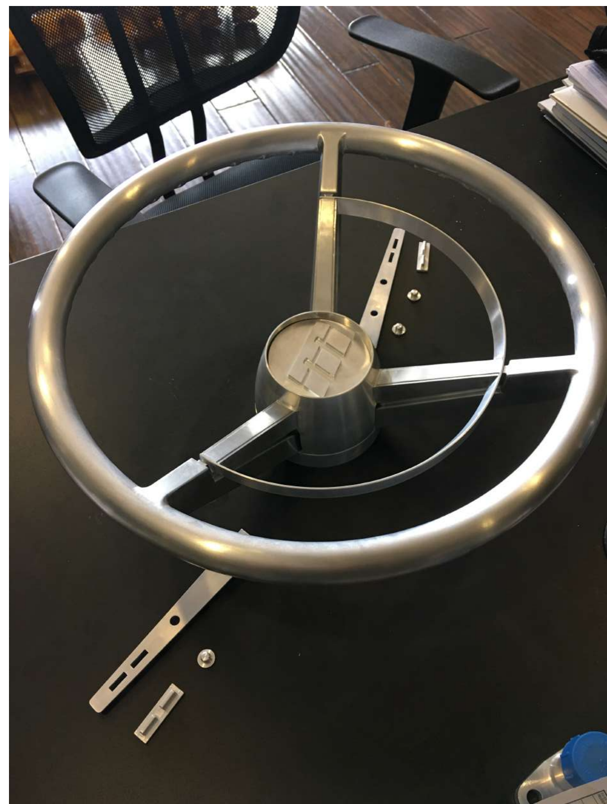
Custom Steering Wheel Design with hidden controls on the back.
